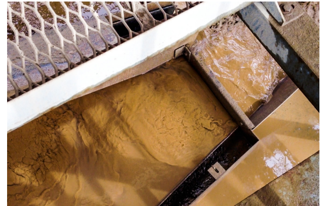
LOAD ZONE BAFFLE SETTLES FINES
