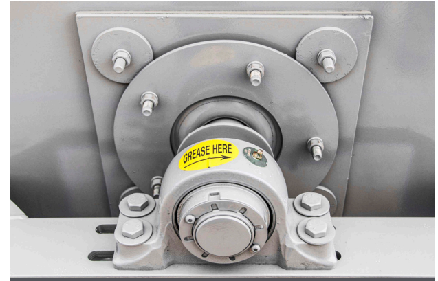
SLINGER PROTECTS LOWER BEARING
