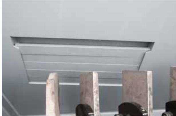
ADJUSTABLE OVERFLOW GATE
