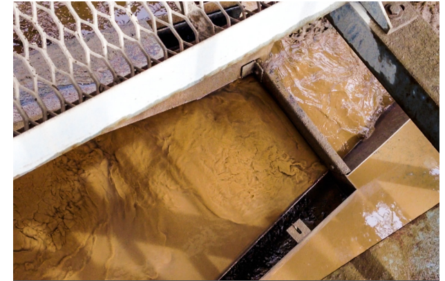
LOAD ZONE BAFFLE SETTLES FINES
