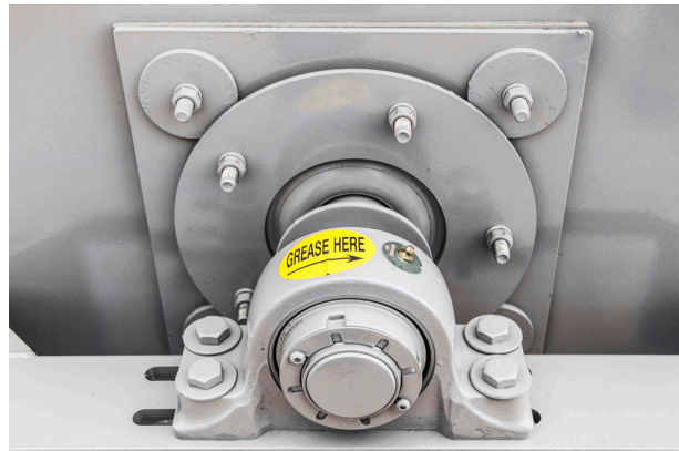
SLINGER PLATE PROTECTS LOWER BEARING
