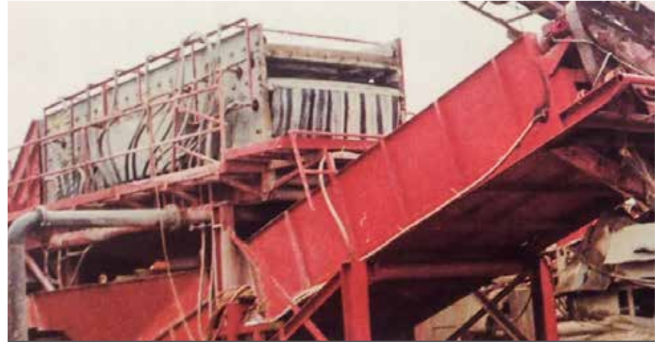
SEMI-PORTABLE WASH PLANT
