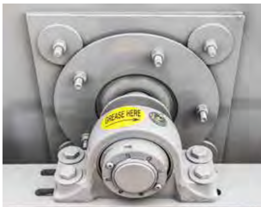
SLINGER PROTECTS LOWER BEARING
