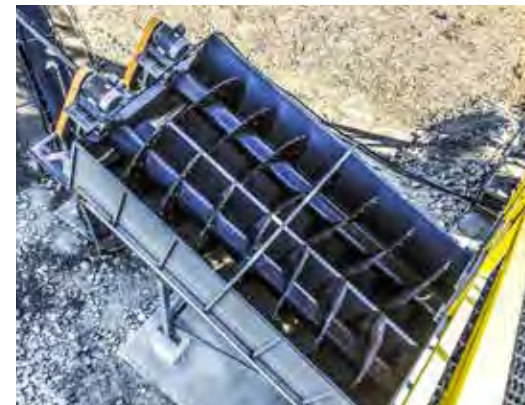
TWIN DEWATERING SCREWS
