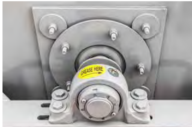
SLINGER PLATE PROTECTS LOWER BEARING
