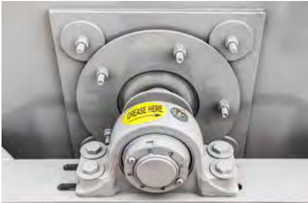
SLINGER PROTECTS LOWER BEARING
