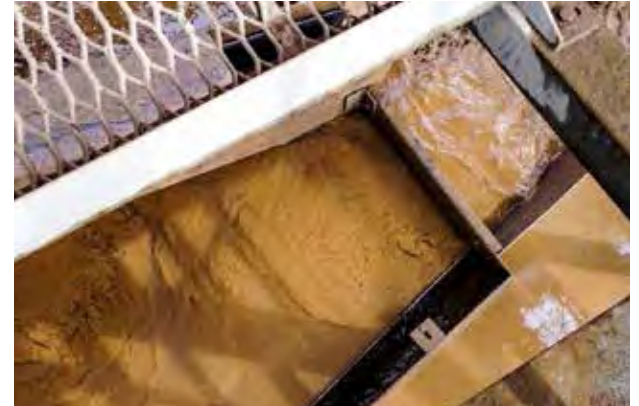
LOAD ZONE BAFFLE SETTLES FINES
