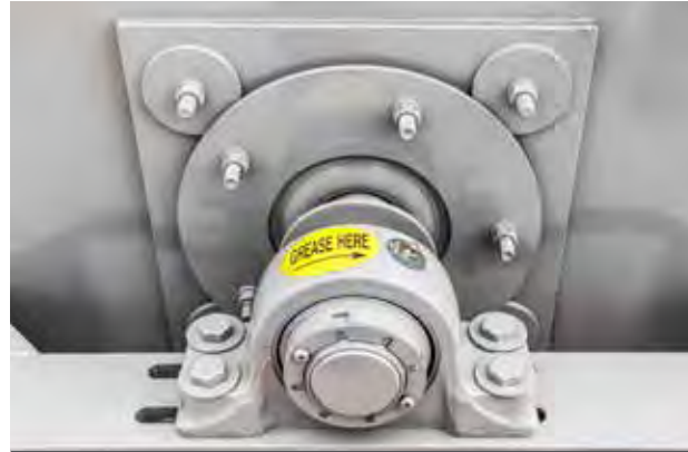
SLINGER PROTECTS LOWER BEARING
