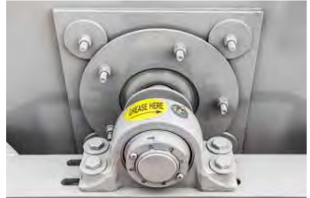
SLINGER PROTECTS LOWER BEARING
