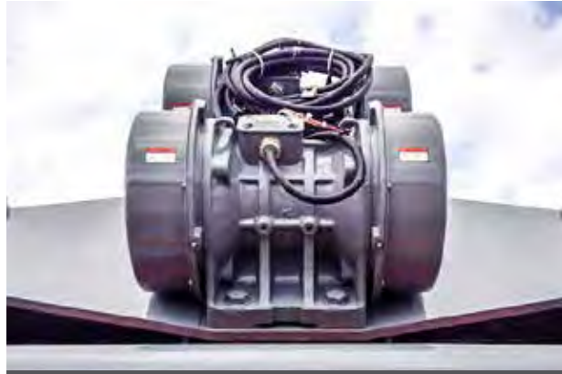
DUAL ELECTRICAL VIBRATORS
