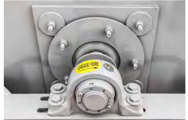
SLINGER PROTECTS LOWER BEARING
