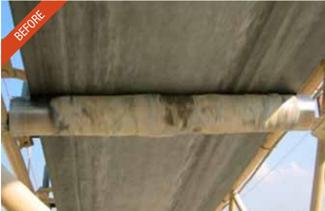
STICKY MATERIAL CLINGING TO STEEL RETURNS CAUSES BELT MIS-TRACKING
