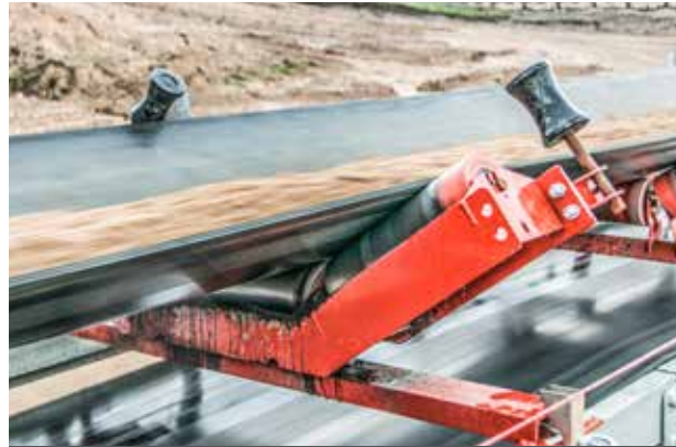
SELF-ALIGNING TROUGHING IDLERS
