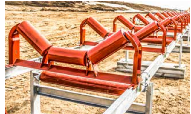
TROUGHING IDLERS ATTACH WITH J-BOLTS
