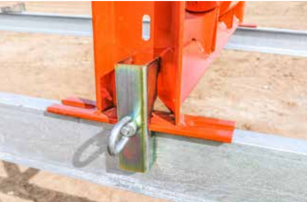
TOOLLESS IDLER INSTALLATION
