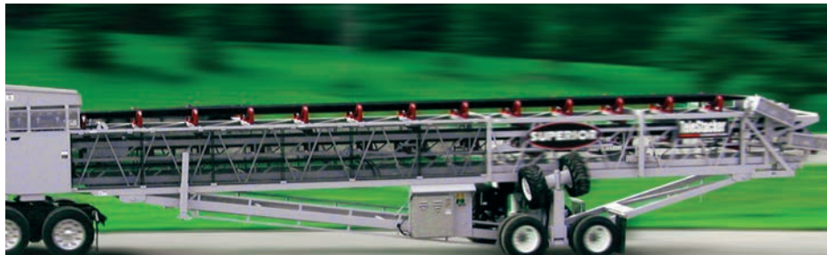
FD AXLE TRANSFERS FROM ROAD TO STOCKPILE MODE IN SECONDS
