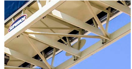
C/ STINGER CROSS BRACING
