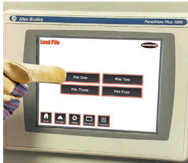
TOUCH SCREEN REACTS TO GLOVE CONTACT
