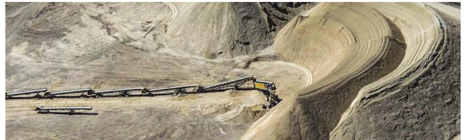
RADIAL WINDROW STOCKPILING ACHIEVES IN-SPEC MATERIAL MIX
