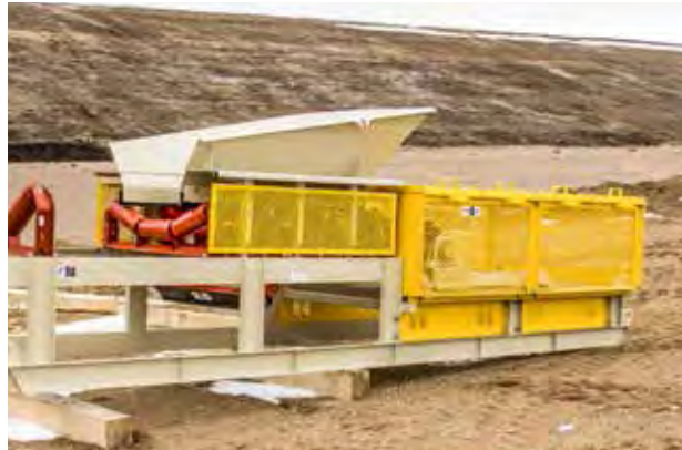
PRE-ASSEMBLED TAIL SECTION
