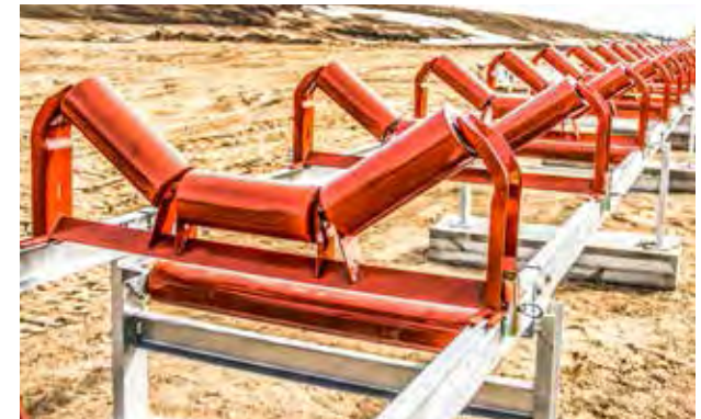
TROUGHING IDLERS ATTACH WITH J-BOLTS
