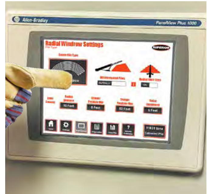
SET PILE PARAMETERS IN VISUAL SETTING SCREEN
