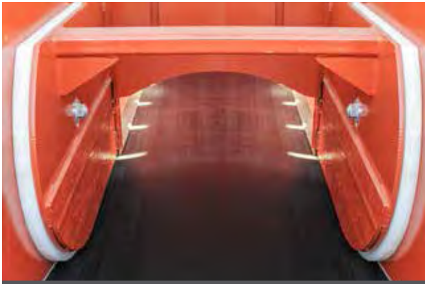
ADJUSTABLE FLOW GATE CONTROLS RATES
