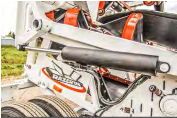
CYLINDER RODS PROTECTED DURING OPERATION
