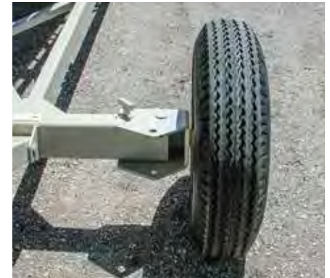
SWIVEL WHEELS FOR ROAD/RADIAL
