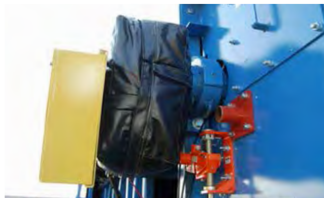
THERMAL SLEEVE INSULATORS
