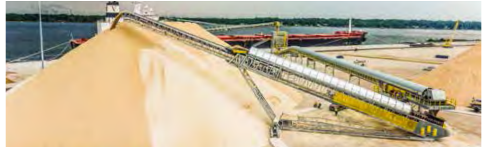
72" X 190' STOCKPILES AT 5,000 TPH
