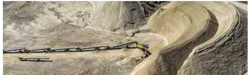
RADIAL WINDROW STOCKPILING ACHIEVES IN-SPEC MATERIAL MIX
